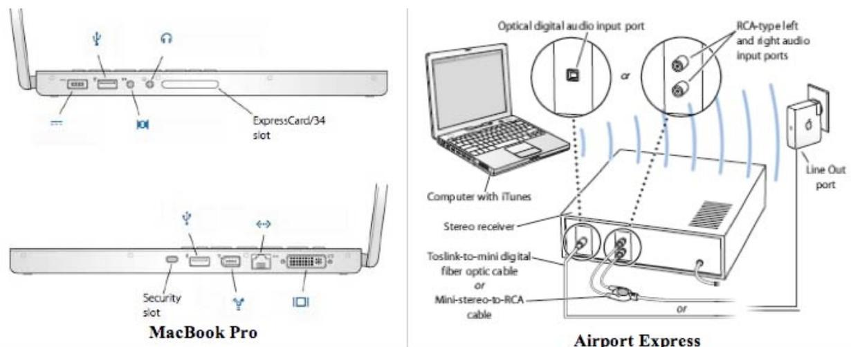
But you see, Apple didn't just take the port and make it just for headsets. They took it up a notch, literally. The audio port is a combo port, meaning that it takes copper *and* fiber type connectors. These jacks provide digital audio out as well as analog audio.
