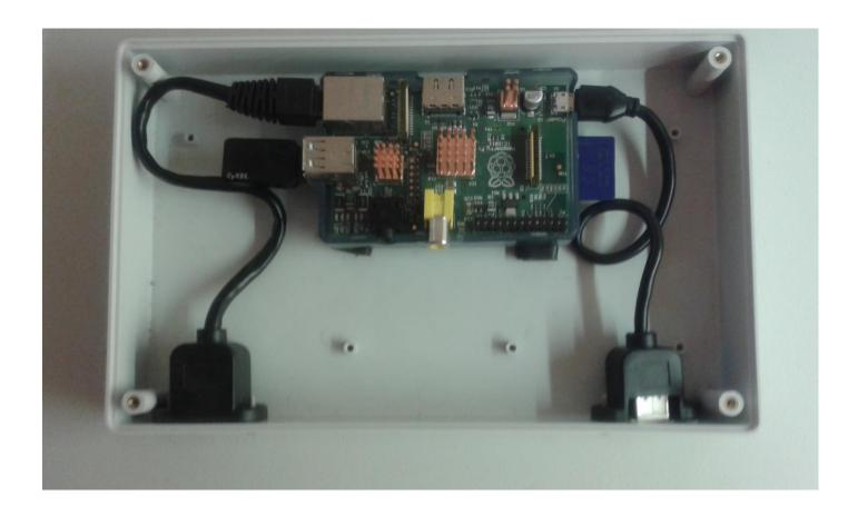
The simple platform is based on a ARM processor. It has a built in 10/100 Mb/s nic and 2 USB2 ports. This doesn't make it unique these days – but what is interesting is the diminutive price tag. Even with the add-on costs, this puts multi-sensor deployments in the reach of even the most cash strapped cash organisations.
